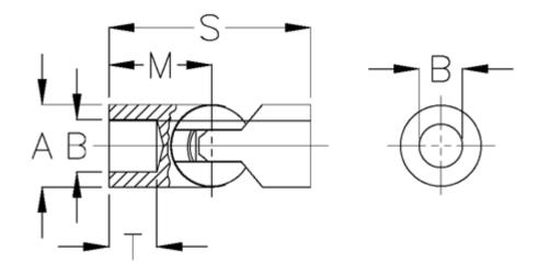
A = 50 B H7 = 25 M = 62.5 Max torque (Nm) = 290 s = 125 T = 30
